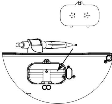
3. The sandblasting tail line of the main engine: there is a sand hose in the tail line of the sandblasting handpiece, and the wear of the hose for a long time may lead to air leakage and sand leakage of the tail line; it needs to be replaced after damage.
