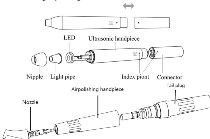
Figure 9 Ultrasonic handpiece and Air polishing handpiece
