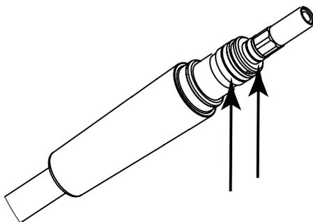
2. Sand pipe at the bottom of the main engine: there is an on-off valve to control the sand powder on and off at the bottom of the main engine, and the sand pipe at the on-off valve may be damaged for a long time; it needs to be replaced after damage.
