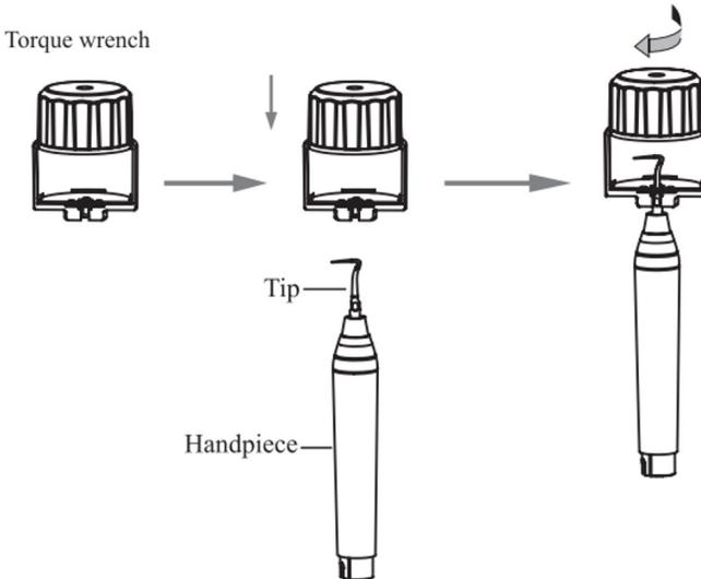
Figure 5 Installation diagram of tip
